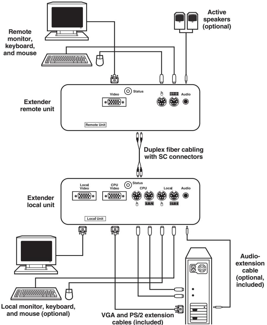
**Figure 4-1. How to install an extender system.**
