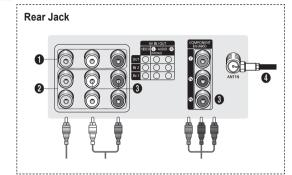
Whenever you connect an audio or video system to your television, ensure that all elements are switched off. Please be sure to match the color coded input terminals and cable jacks.
