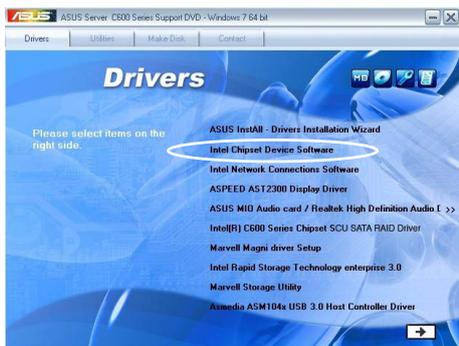
4. The **Intel(R) Chipset Device Software** window appears. Click **Next** to start installation.
