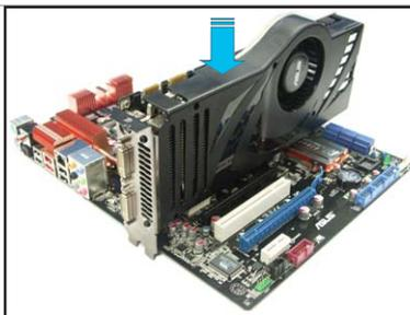
4. Align and firmly insert the SLI bridge connector to the goldfingers on each graphics card. Ensure that the connector is firmly in place.
