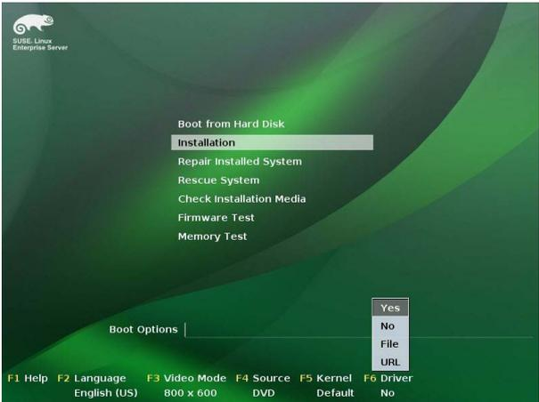
4. Use the USB drive to provide the third-party driver during the OS installation. Type the command `brokenmodules=ahci` in **Boot Options** field, and press `<Enter>`.
