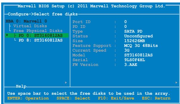
3. Press **<Space>** to select the hard drives to be included in the RAID array. An asterisk (\*) appears in front of the selected hard drive. After selecting all the drives needed for the RAID array, press **<Enter>** to continue.
