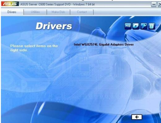
4. When the **Intel® WG82574L Gigabit Adapters Driver** installation wizard appears, click **Next** to start the installation.
