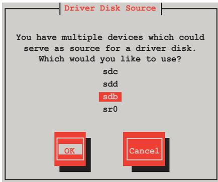
6. Insert the Red Hat® Enterprise RAID driver disk to the USB floppy disk drive, select **OK**, then press <Enter>.
