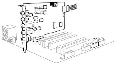
5. Connect the power cable of your power supply unit (PSU) to the power connector of the audio card.
