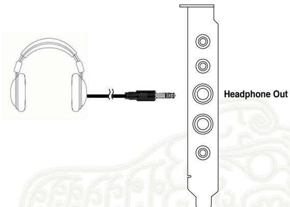
The Headphone Out port has a built-in high-quality amplifier for headphones. Connect your stereo headphones to the headphone output ports on the Xonar Essence ST card.
