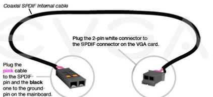
Plug the 2-pin white connector to the SPDIF- pin and the black one to the ground-pin on the motherboard.
