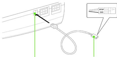
Connect the SPDIF cable into the SPDIF header on the top edge of the graphics card.
