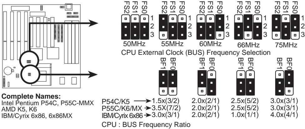
Set the jumpers by the Internal speed of the Intel, AMD, or Cyrix CPU as follows:
