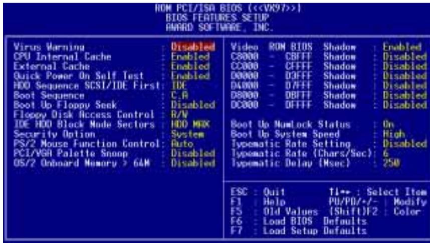
A section at the lower right of the screen displays the control keys you can use. Take note of these keys and their respective uses. If you need information on a particular entry, highlight it and then press the <F1> key. A pop-up help menu will appear to provide you with the information you need. To load the last set values, press the <F5> key. <F6> and <F7> load the BIOS default values and Setup default values, respectively.
