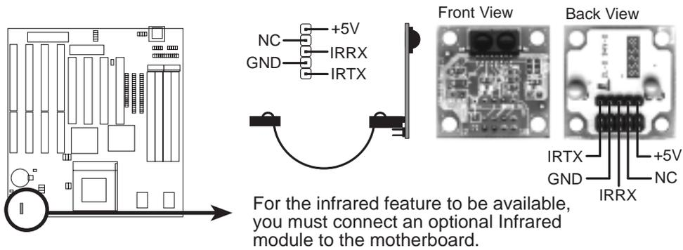
**Infrared Module Connector**
