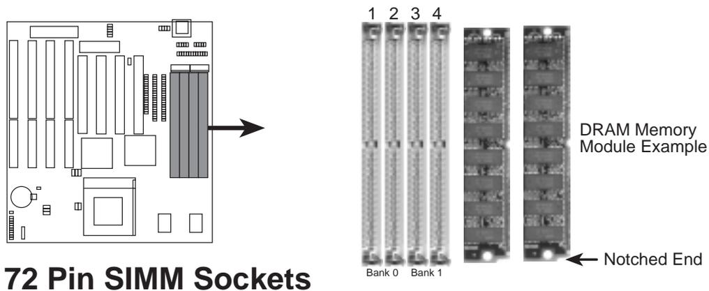
2. Press the memory module firmly into place starting from a 45 degree angle making sure that all the contacts are aligned with the socket.
