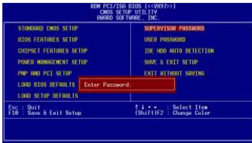
To implement the password protection, specify in the “Security Option” field of the BIOS Features Setup screen when the system will prompt for the password. If you want to disable either password, press the <Enter> key instead of entering a new password when the “Enter Password” prompt appears. A message confirms the password has been disabled.
