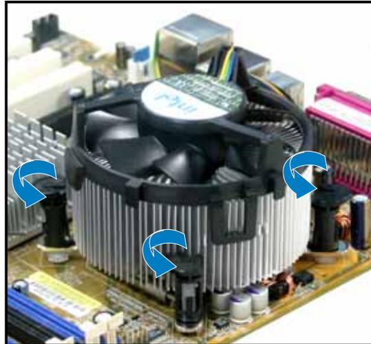
3. Pull up two fasteners at a time in a diagonal sequence to disengage the heatsink and fan assembly from the motherboard.
