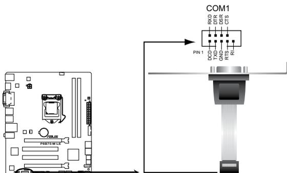
**P8B75-M LE Serial port (COM1) connector**
