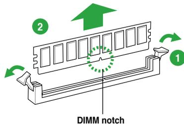
2. Remove the DIMM from the socket.
