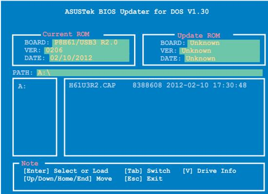
3. Press <Tab> to switch between screen fields and use the <Up/Down/Home/End> keys to select the BIOS file and press <Enter>. BIOS Updater checks the selected BIOS file and prompts you to confirm BIOS update.
