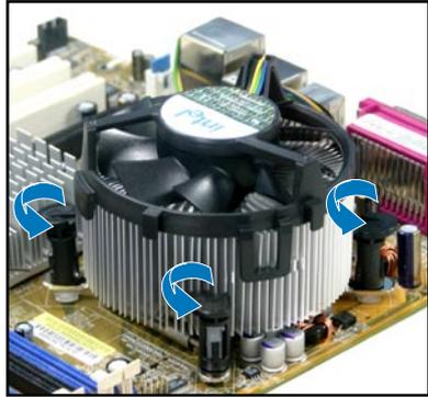
3. Pull up two fasteners at a time in a diagonal sequence to disengage the heatsink and fan assembly from the motherboard.
