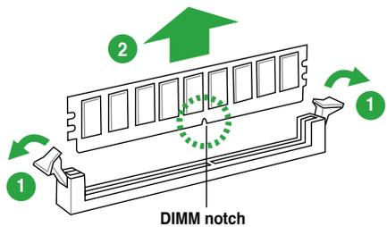
2. Remove the DIMM from the socket.
