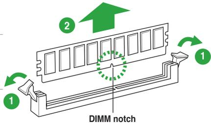
2. Remove the DIMM from the socket.
