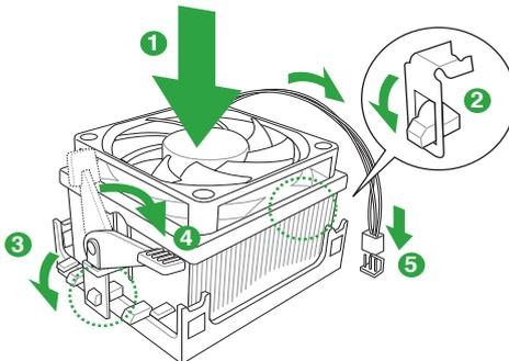
3. Align the other end of the retention bracket to the retention module base. A clicking sound denotes that the retention bracket is in place.
