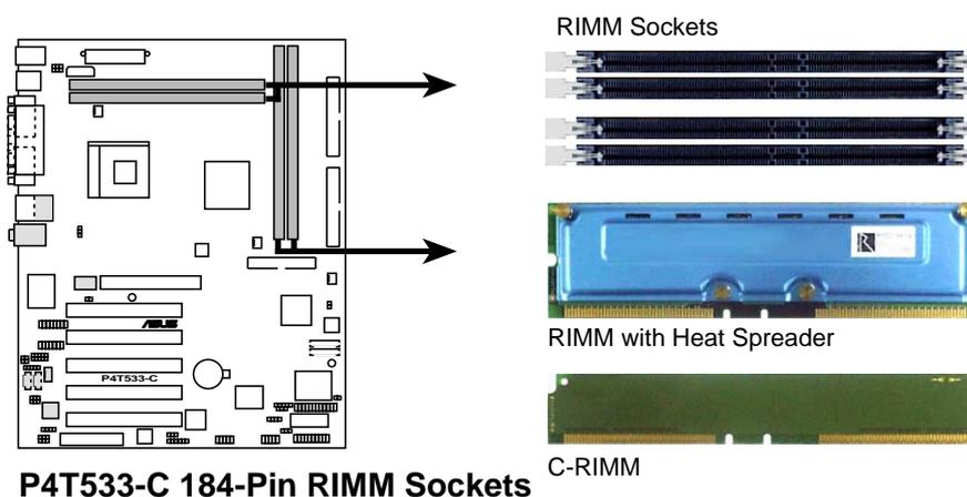
1. Make sure that the notch keys in the module are aligned with the small ribs inside the RIMM sockets.
