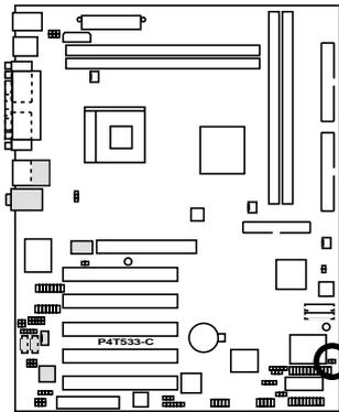
**TIP:** If the case-mounted LED does not light, try reversing the 2-pin plug.
