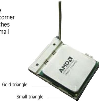
5. When the CPU is in place, push down the socket lever to secure the CPU. The lever clicks on the side tab to indicate that it is locked.
