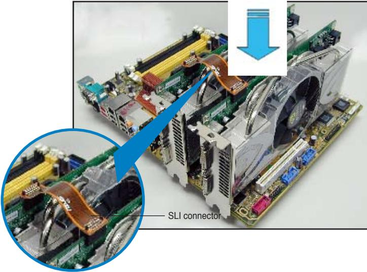
6. When installing two VGA cards using a 20-pin ATX PSU with sufficient+12v capability, we recommend that you connect the auxillary power source from the power supply to the graphics card. Refer to the PSU documentation for dual VGA power requirements.
