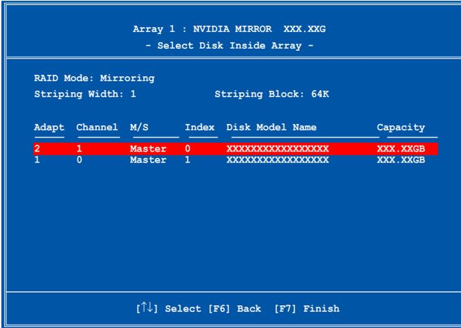
3. Use the up or down arrow keys to select a RAID array to rebuild, then press <F7>. The following confirmation message appears.
