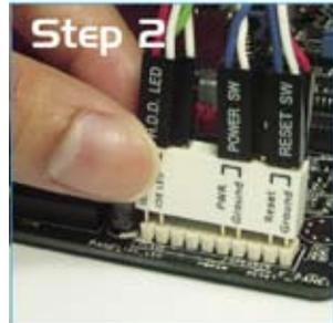
When installed, the Q-connector appears as shown.
