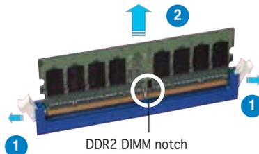
2. Remove the DIMM from the socket.
