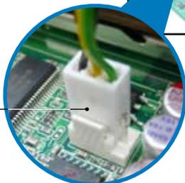
4. Repeat steps 1 to 3 to install the other heatsink if you have installed a second CPU, then connect the fan cable to the 4-pin connector labeled CPU\_FAN1.
