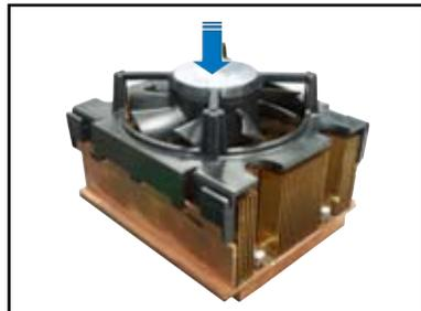
2. Use a Phillips screwdriver to tighten the four heatsink screws in a diagonal sequence.
