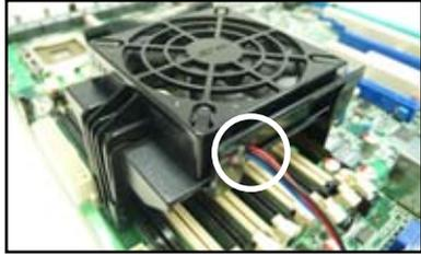
5. Connect the fan cable to the 4-pin connector labeled FBD\_FAN1.
