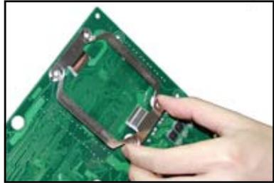
5. If you installed a second CPU, repeat steps 2 to 4 to install the CEK spring to the CPU2 heatsink holes. The CEK springs appear as shown when installed.
