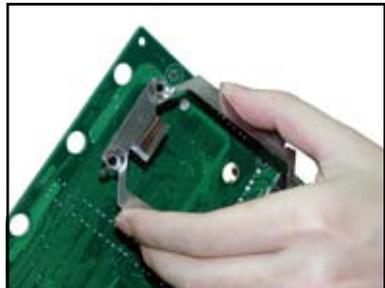
3. Press the upper spring hooks inward, then insert to the upper CPU heatsink holes until they snap in place.
