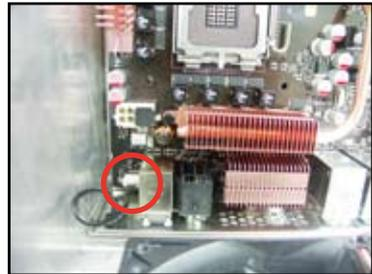
5. This photo shows the LCD Poster installed. Place the device wherever you can monitor the screen.
