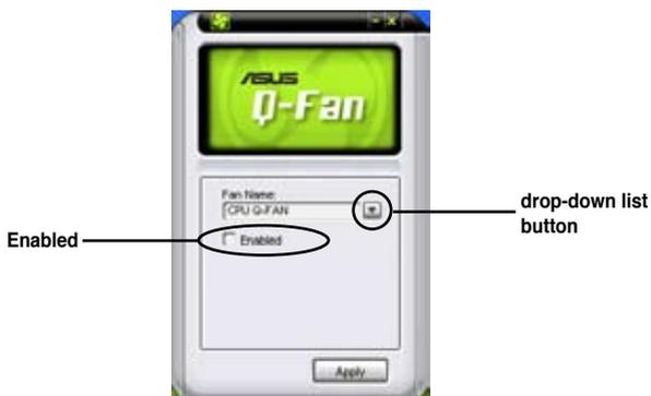
**Profile** list appears after clicking the **Enabled** box. Click the drop-down list button and select a profile. **Optimal** mode makes the fans adjust speed with the temperature; **Silent** mode minimizes fan speed for quiet fan operation; **Performance** mode boosts the fan to achieve maximal fan speed for the best cooling effect.
