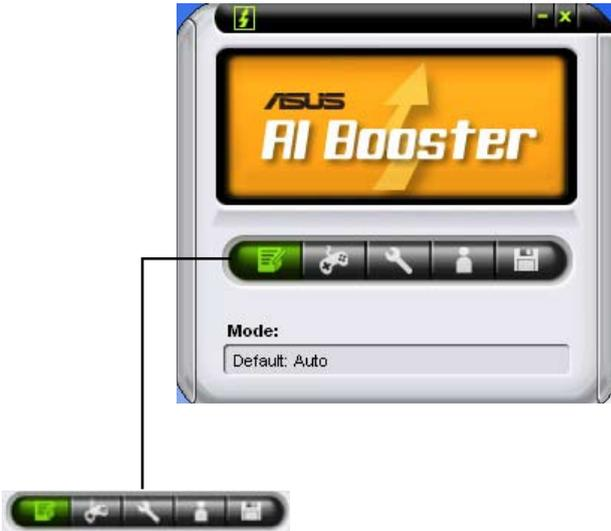
The options on the taskbar allow you to use the default settings, adjust CPU/ Memory/PCI-E frequency manually, or create and apply your personal overclocking configurations.
