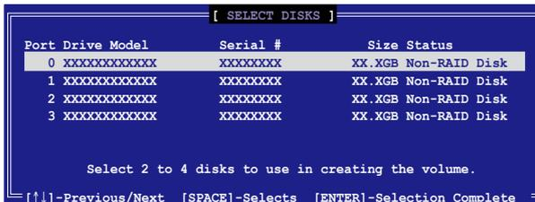
5. Use the up/down arrow key to highlight a drive, then press <Space> to select. A small triangle marks the selected drive. Press <Enter> after completing your selection.
