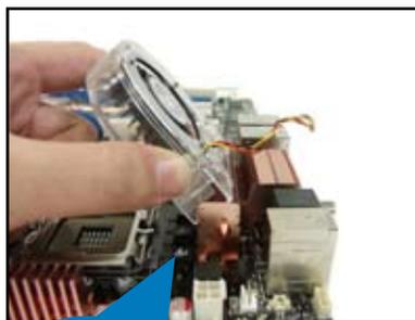
3. Carefully push down the fan until it snugly fits the heatsink, then connect the fan cable.
