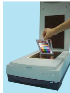
Positioning the target on the upper scan bed
