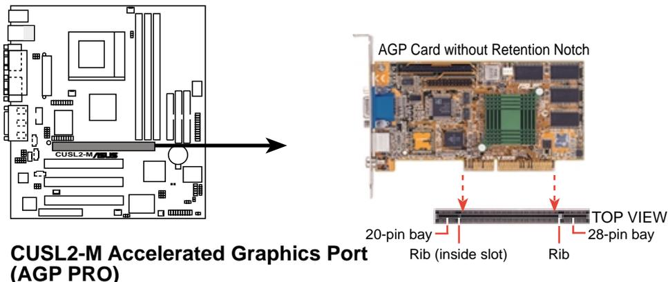
**NOTE:** Disable the integrated graphics controller (see **Onboard VGA** in **4.4.1 Chip Configuration**) when using an add-on graphics card.
