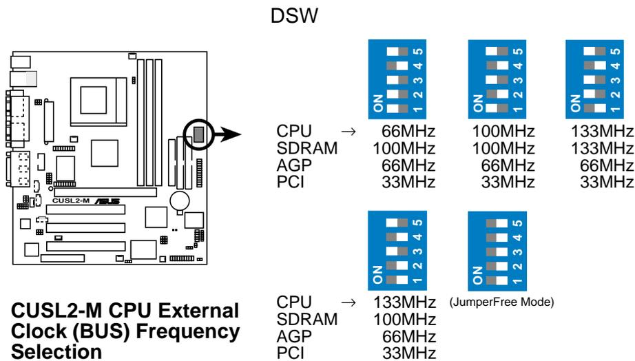
**NOTE:** If your processor does not have a locked Frequency Multiple, you must use **CPU Core:Bus Freq. Multiple** in *4.4 Advanced Menu* to set the Frequency Multiple. If the Frequency Multiple is locked, setting the Frequency Multiple in BIOS setup will have no effect.
