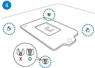
To uninstall the CPU heatsink and fan assembly
