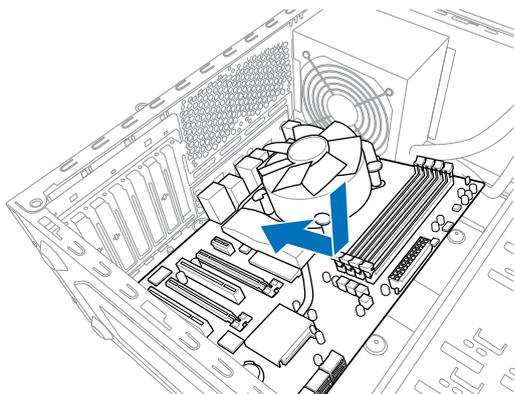
3. Place six screws into the holes indicated by circles to secure the motherboard to the chassis.
