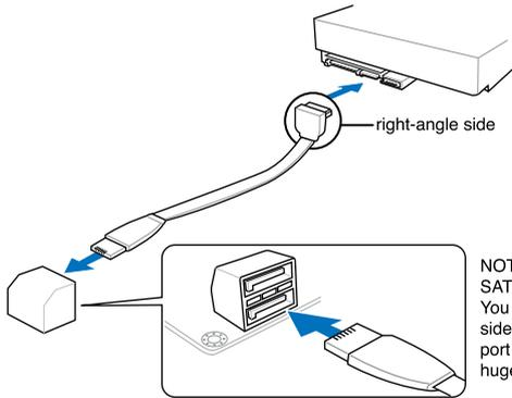
NOTE: Connect the right-angle side of SATA signal cable to SATA device. You may also connect the right-angle side of SATA cable to the onboard SATA port to avoid mechanical conflict with huge graphics cards.
