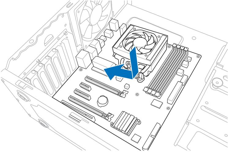
3. Place nine screws into the holes indicated by circles to secure the motherboard to the chassis.
