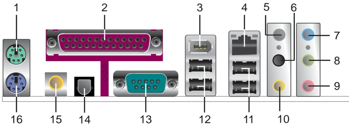
1. **PS/2 mouse port.** This green 6-pin connector is for a PS/2 mouse.
