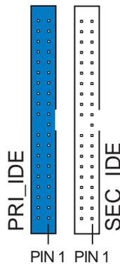
**NOTE:** Orient the red markings (usually zigzag) on the IDE ribbon cable to PIN 1.
