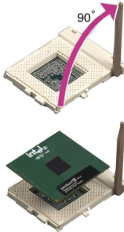
**CAUTION!** The CPU fits only in one orientation. Do not force the CPU into the socket to prevent bending the pins and damaging the CPU. If the CPU does not fit completely, check its orientation or check for bent pins.
