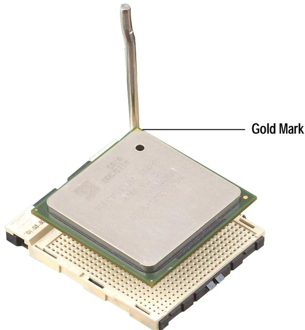
5. When the CPU is in place, press it firmly on the socket while you push down the socket lever to secure the CPU. The lever clicks on the side tab to indicate that it is locked.
