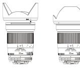
The hood has a bayonet system, which guarantees speedy, efficient, safe and precise installation and will help you take shots that are free of flaring and ghosting. Allign the attachment reference point on the hood with the reference point on the lens. Push the hood onto the lens and turn the hood to the right until it makes a clicking sound.
