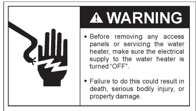
1. Before beginning turn "OFF" the electric power supply to the water heater.
