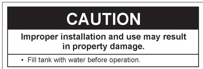
Never use this water heater unless it is completely full of water. To prevent damage to the tank and heating element, the tank must be filled with water. Water must flow from the hot water faucet before turning "ON" power.
