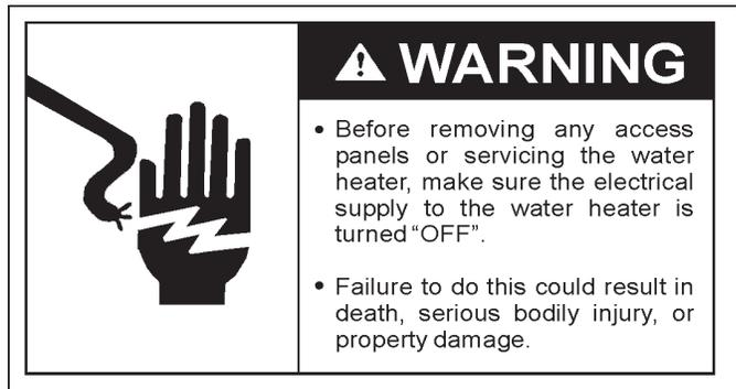
1. Before beginning turn "OFF" the electric power supply to the water heater.
