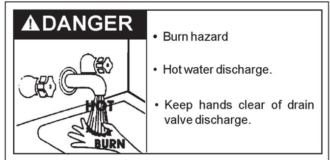
The water passing out of the drain valve may be extremely hot. To avoid being scalded, make sure all connections are tight and that the water flow is directed away from any person.
