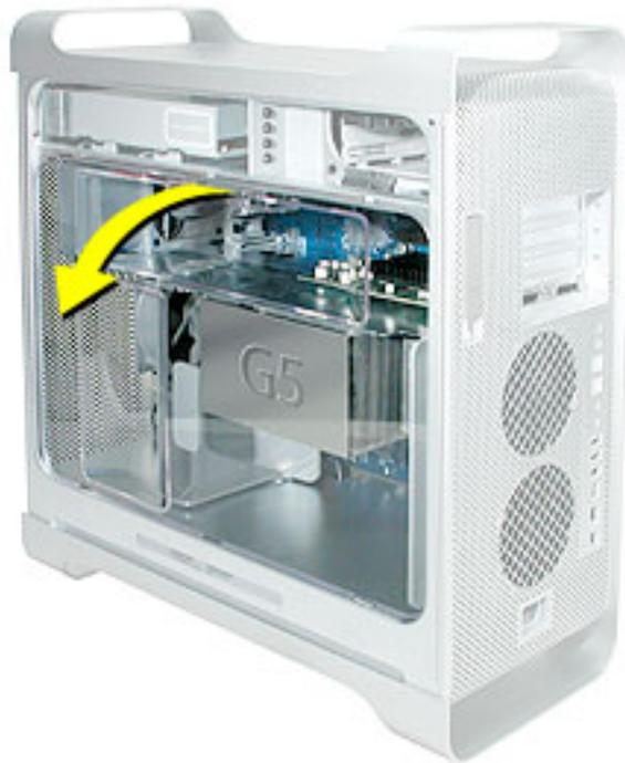
**Important:** Always remember to replace the air deflector after you have finished working inside your computer. The Power Mac G5 computer will not function properly if the air deflector is not replaced.
