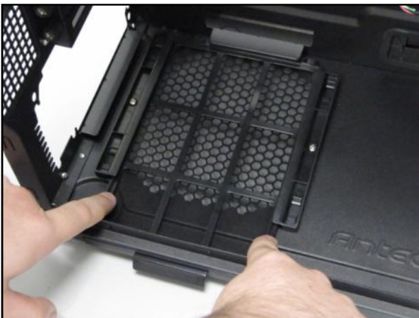
Push down on the ends of the filter to unlock it.
