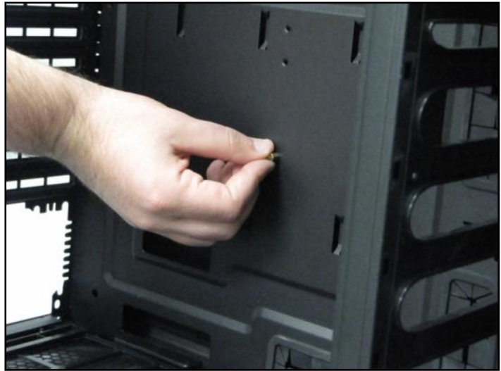
Installing the motherboard standoffs.
