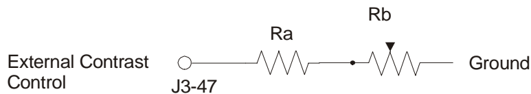
Figure 2–10. External Contrast Adjustment for LCD Panels
