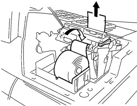
B: Installation using the **[RF]** key
