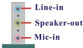
**Line In (Blue)** This port is for connecting an external audio device such as a CD player, tape player or other audio devices that provide an audio input. When the Super 5.1 Channel Audio Effect is enabled, your rear speaker function will be enabled with this port.
