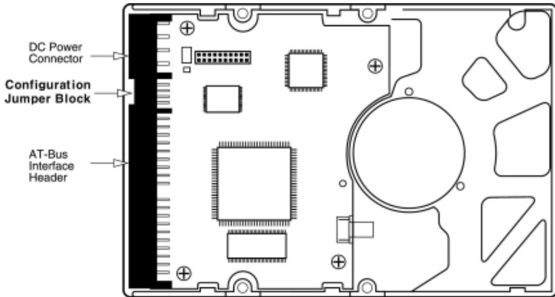
Figure 4-5 Jumper Pin Locations on the Drive PCBA
