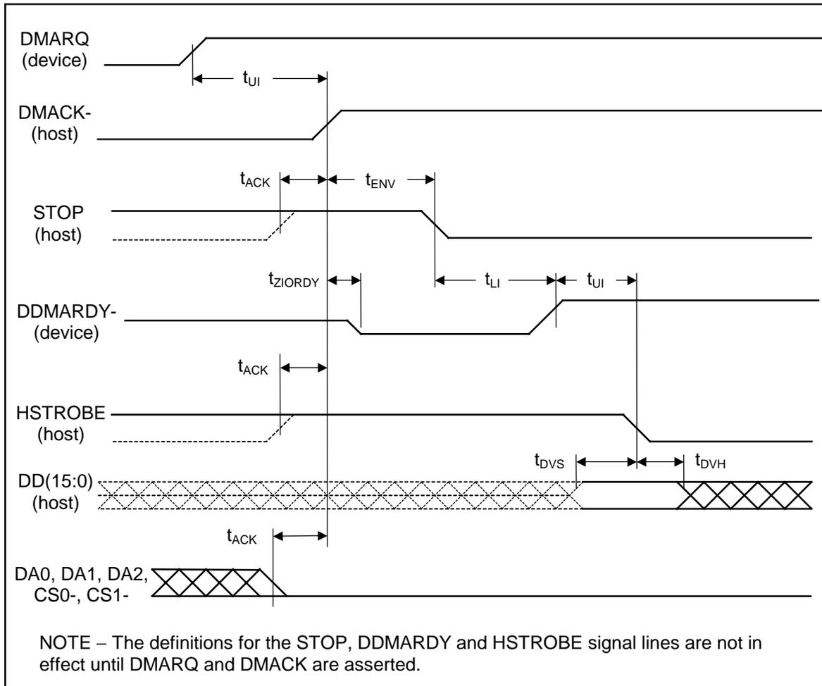
**Figure 6-9** Initiating an Ultra DMA data out burst
