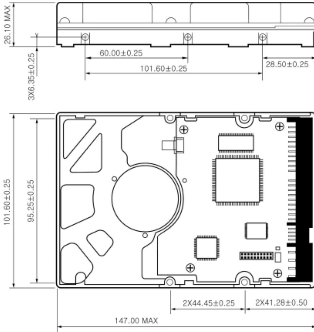
**Figure 4-2** Mounting Dimensions (in Millimeters)
