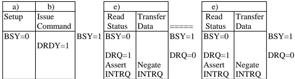
If Error Status is presented, the drive is prepared to transfer data, and it is at the host's discretion that the data is transferred.
