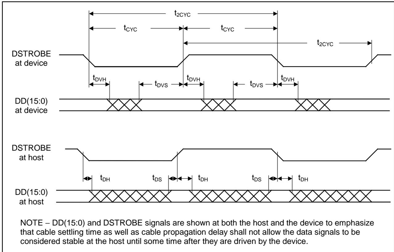
**Figure 6-5** Sustained Ultra DMA data in burst
