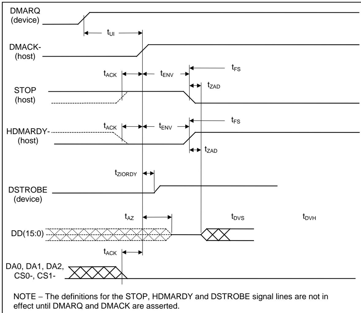
Figure 6-4 Initiating an Ultra DMA data in burst
