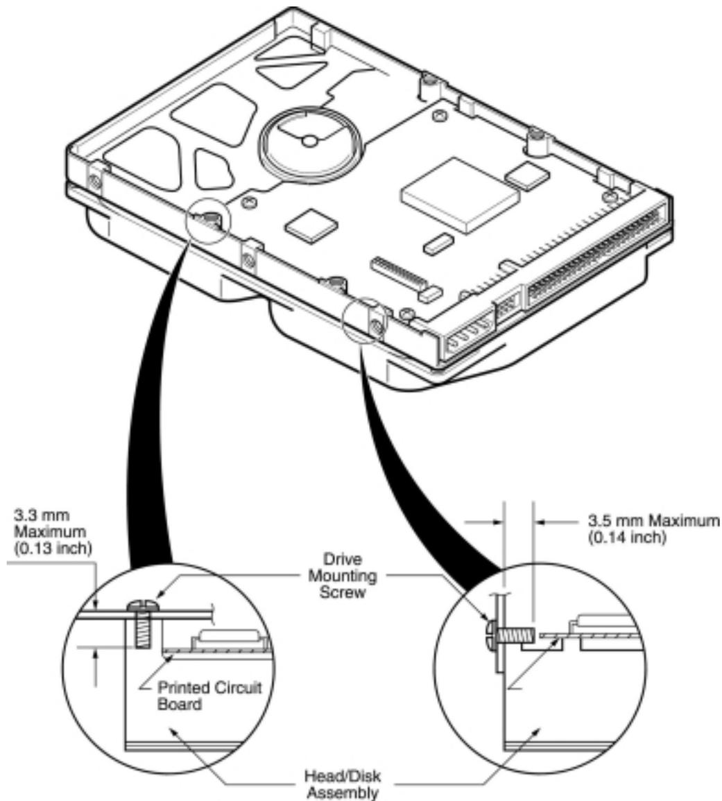
Figure 4-3 Mounting-Screw Clearance
