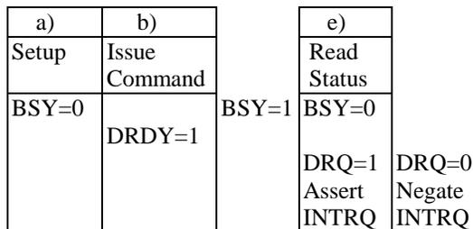
Although DRQ=1, there is no data to be transferred under this condition.
