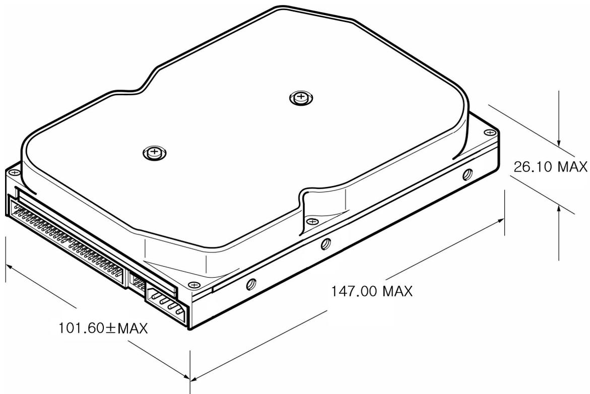
**Figure 4-1** Mechanical Dimension
