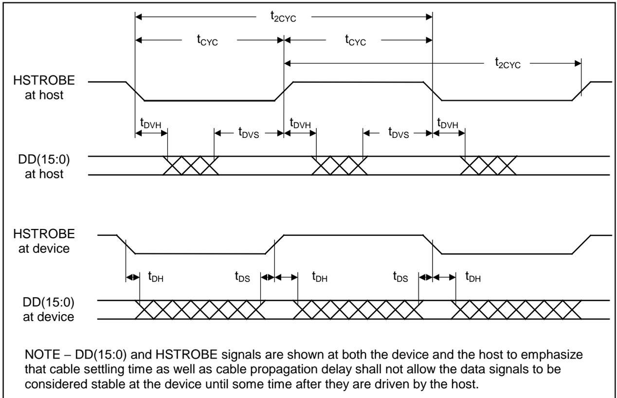
Figure 6-10 Sustained Ultra DMA data out burst
