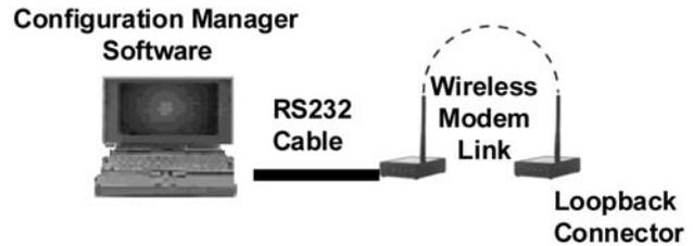
**Fig. 1 — Loopback Configuration**
