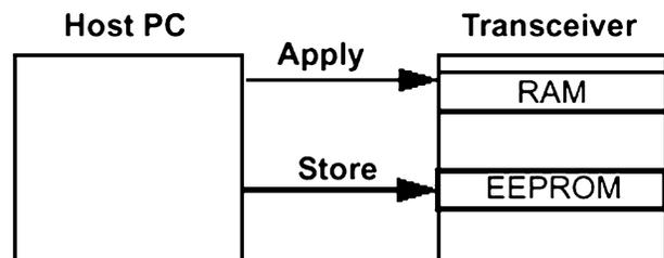
Fig. 12 — Setting Storage Process
