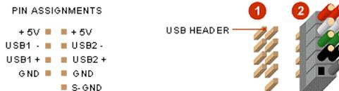
**Diagram 1:** On most motherboards, the USB header/pin-out consists of 9 pins arranged in 2 rows; and each header allows for 2 USB connections (i.e. USB1 and USB2). Normally, the pins for USB1 and USB2 are in separate rows.
