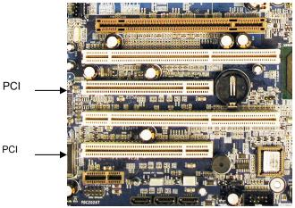
Note: The AEMK35CB PCI controller connects to a PCI bus slot.
