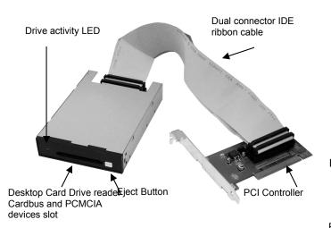
Connect the other end of the dual connector IDE ribbon cable to the IDE connector on the Desktop Card Drive reader.
