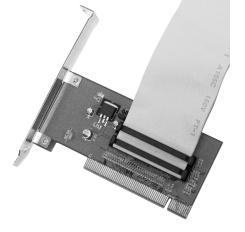
3. Plug-in the PCI controller on a PCI bus slot.
