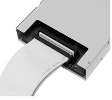
2. Connect one end of the dual connector IDE ribbon cable to the IDE connector on the PCI controller.
