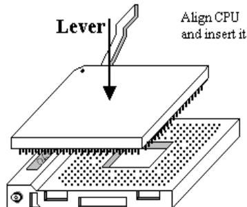
**Figure 2-2. Install the CPU into socket A**
