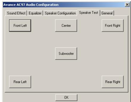
This menu item can let you test the speaker position is correct or wrong, you can check each speaker is sound correctly or poor quality.
