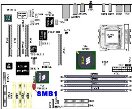
This header is reserved for the system management bus (SM-Bus). The SM-Bus is a specific implementation of an I<sup>2</sup>C bus. I<sup>2</sup>C is a multi-master bus, this means that multiple chips can be connected to the same bus and each one can act as a master by initiating a data transfer. If more than one master simultaneously tries to control the bus, an arbitration procedure decides which master gets priority. You can connect the devices which utilizes the SM-Bus.
