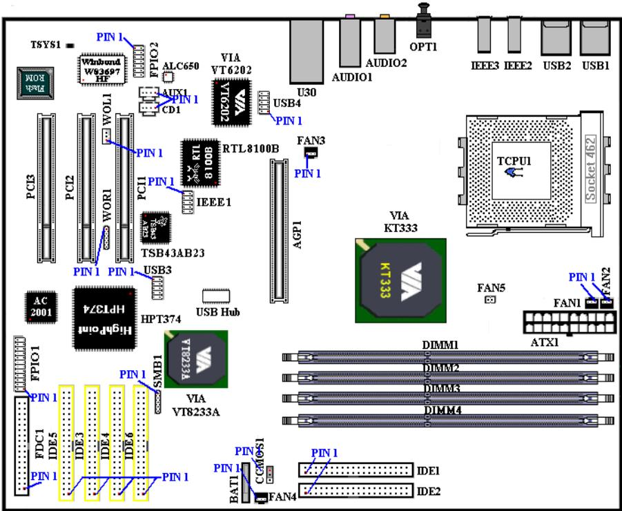
**Figure 2-7. All connectors and headers for the AT7**
