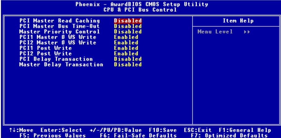
Figure 3-5E. CPU & PCI Bus Control Screen
