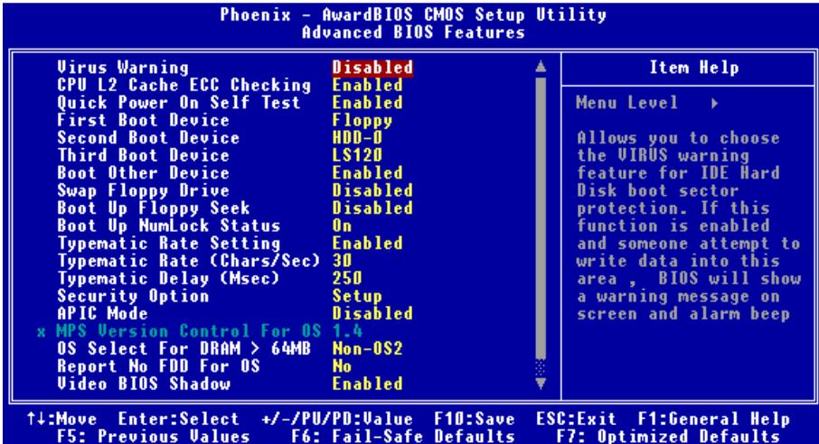
Figure 3-4A. Advanced BIOS Features Setup Upper Screen
