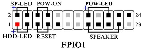
**FPIO1 (Pin 1 & 3): HDD LED Header**
