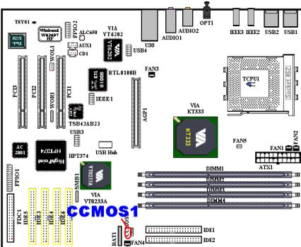
Jumper CCMOS1 used to discharge CMOS memory. When you install the motherboard, make sure this jumper is set to normal operation (pin 1 and 2 shorted). See figure below.
