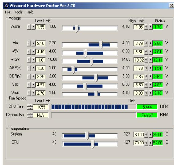
This screen shows the hardware monitor system screen. It shows information about system temperature, voltages and fan speed. Some items can let you set the warning range; you can optimize values by setting them in accordance your system.
