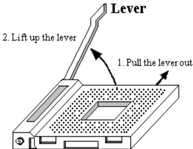
**Figure 2-1. Socket A and open its lever**
