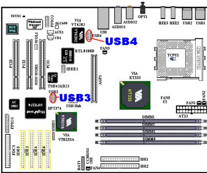
These headers are for connecting the additional USB port plugs. Each connector can provide two additional USB plugs. Which means, total you can get two additional USB plugs from each connector. You can use the special USB port expansion cable to connect it (the cable come with the metal plate can fix on the back panel of computer chassis).
