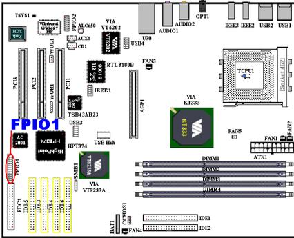
FPIO1 are for switches and indicators for the chassis’s front panel, there are several functions that come from this header. You have to watch the pin position and the orientation, or you may cause LED not light up. Figure below shows you the FPIO1 functions of the pins.
