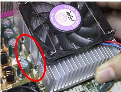
Insert the heatsink left side fix plate into the processor socket left side fix hooks. Make sure the fit is very tight. Check the photo on the left.
