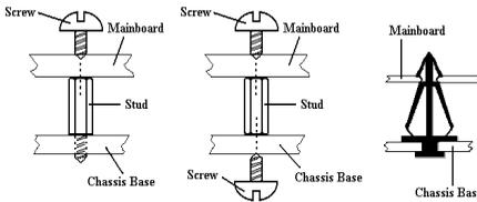
**Figure 2-4. The way we fixed the motherboard**
