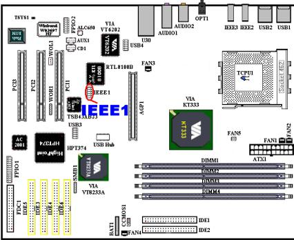
This header is reserved for connection to the **ABIT Media XP** product (**Optional**). The **Media XP** can provide the total solution for the front panel connections. It provided a various function, like a: SD/MS/CF card reader, USB 2.0/IEEE 1394 connectors, S/PDIF-Out connector and MIC/Earphone connectors. They all designed on one 5.25" diskette size panel, can fit on the chasses front panel 5.25" diskette slot.
