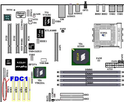
This 34-pin connector is called the “*floppy disk drive connector*”. You can connect a 360K, 5.25”, 1.2M, 5.25”, 720K, 3.5”, 1.44M, 3.5” or 2.88M, 3.5” floppy disk drive.
