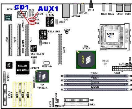
These connectors connect to the audio output of internal CD-ROM drive or add-on card.
