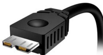
The USB 3.0 Micro-B connector is basically a USB 2.0 Micro-B connector with an extension holding 5 extra pins. The port on the My Book 3.0 is designed for this connector. You can also use a USB 2.0 cable with the My Book 3.0, but the drive will only operate at USB 2.0 speeds.
