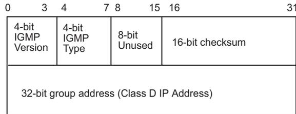
**Figure 5-2** Format of an IGMP Version 1 Message
