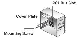
Remove the Acoustic Edge™ Sound Card from the anti-static bag. Align your sound card with the selected PCI Bus-Slot and firmly push it into the slot. Be sure the sound card is aligned properly and fits snugly into the slot
