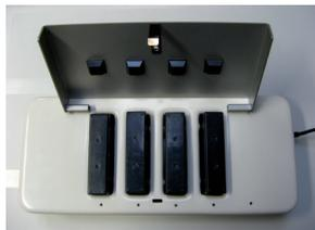
Open the cover of the battery charger. The charger has four compartments to recharge the four batteries simultaneously. The four LEDs
