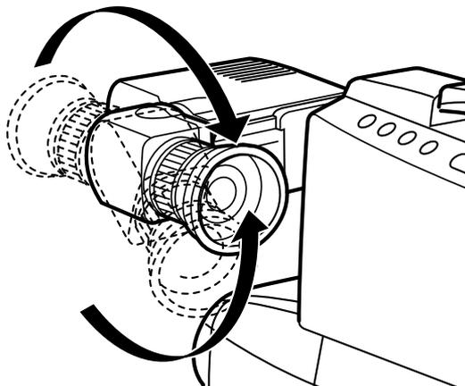
**Caution:** Do not force the eyepiece to rotate completely around. This will damage the eyepiece and/or the camcorder.
