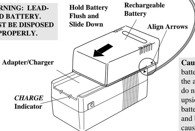
**Caution:** When a battery is attached to the adapter/charger, do not turn them upside down. The battery may fall off and be damaged or cause injury.
