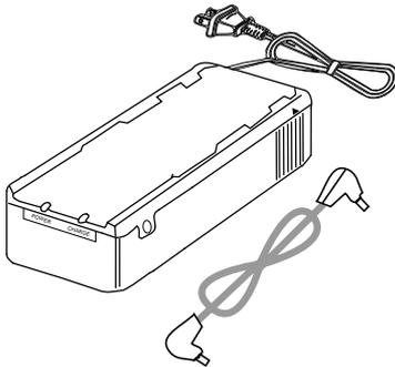
This adapter/charger operates on 100-240 volts, 50/60 Hz, so it can be used almost anywhere in the world to power your camcorder and recharge the EP096FS battery supplied with your camcorder.
