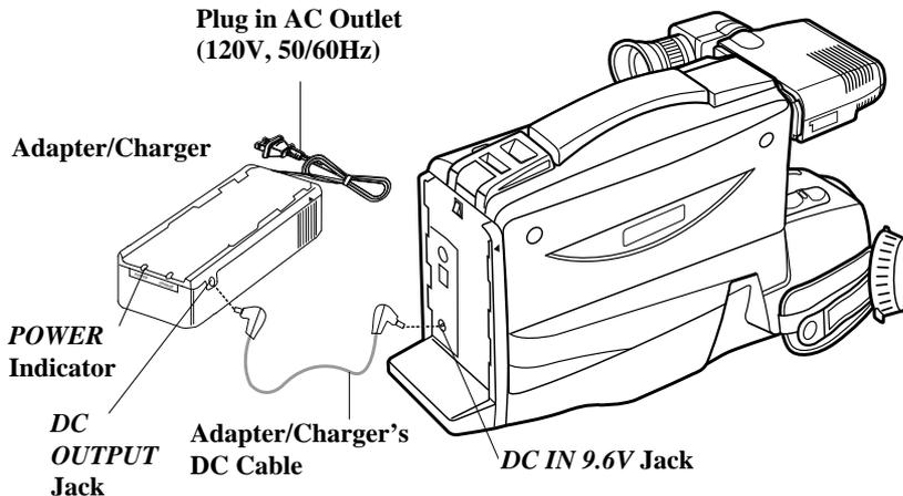
1. Connect one end of the adapter/charger's cable to the adapter/charger's *DC OUTPUT* jack and the other end to the *DC IN 9.6V* jack on the back of the camcorder.
