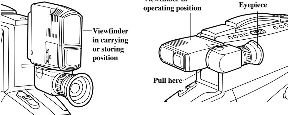
**Caution:** Pulling on the eyepiece may cause damage to the camcorder.
