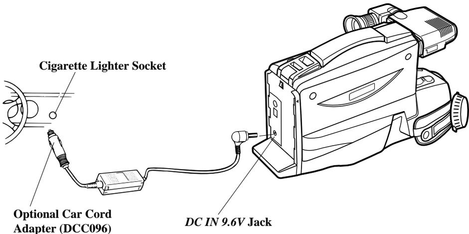
1. Remove the adapter/charger's DC cable or battery from the camcorder, if either is attached.
