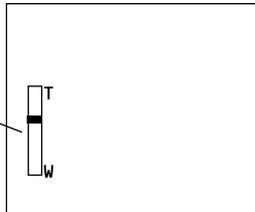
When *DISPLAY* is pressed so the display appears in the viewfinder and the power zoom button is pressed, the zoom level is displayed in 10 steps for several seconds.
