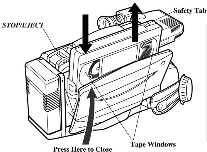
**Caution:** Insert cassette with safety tab facing up and tape windows facing out. Cassette should slide easily into the compartment. **Gently push the cassette down until it locks in place.**
