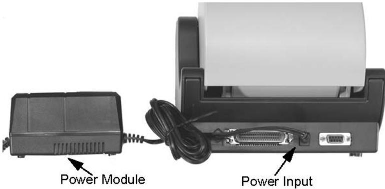
1. Plug the output of the power module provided with the printer into the connector on the rear panel.
