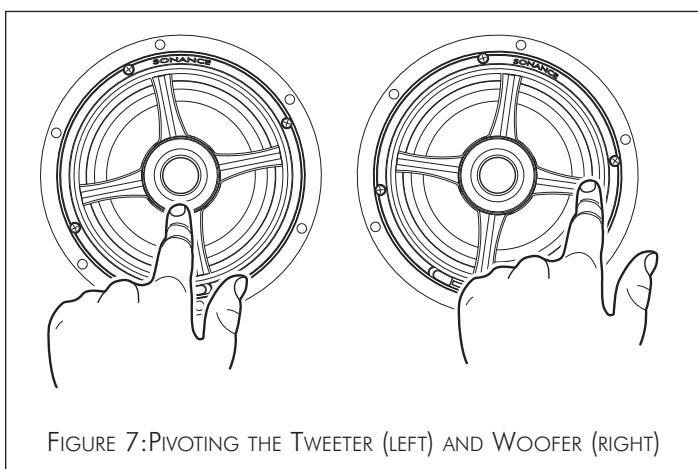
FIGURE 7:PIVOTING THE TWEETER (LEFT) AND WOOFER (RIGHT)
