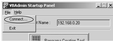
If the connection is disconnected after the VB Admin Startup Panel has started up, choose Connect from the File menu. The Server Setting dialog box then appears.
