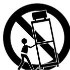
Quick stops, excessive force, and uneven surfaces may cause the equipment and cart combination to overturn.
