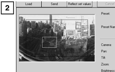
Click the Send button. Check the Status List to be sure the values were sent correctly. Then when the Reflect set values button is clicked, the values will be reflected in the VB101.
