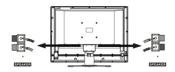
Connect the speaker audio cable to the external speaker output jack on the unit matching the "+" and "-" ends of the cable.
