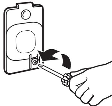
3. Turn bulb counterclockwise. Replace the bulb with a 10-watt appliance bulb only. Replace the cover and secure with the screw.
