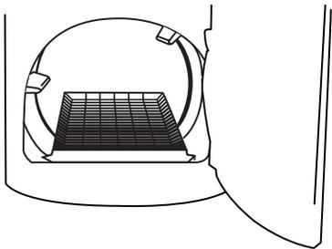
3. Place wet items on top of the drying rack. Allow space around items for air to circulate. The drying rack does not move, but the drum will rotate; be sure to leave adequate clearance between items and the inside of the dryer drum. Make sure items do not hang over the edges or between drying rack grille.
