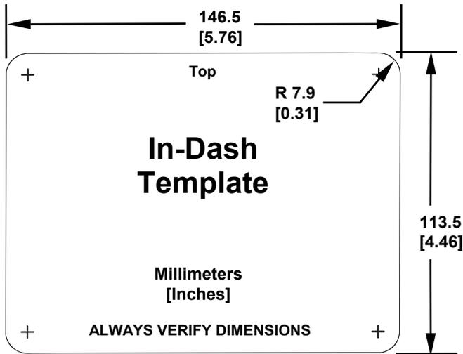
**In-dash mounting template for FishEasy 250DS, showing dimensions. The preceding figure is *not* printed to scale. A scaled template is available for free download from our web site, [www.eaglesonar.com](http://www.eaglesonar.com).**
