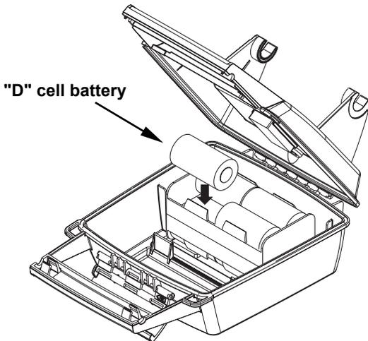
**Install batteries in power case battery adapter.**
