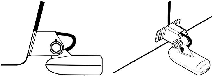
**Route cable over bolt and through bracket. Side view (left) and shown from above (right).**
