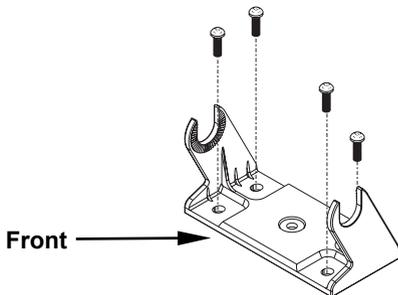
**Install the gimbal bracket. Orient the bracket so the arms slope toward the front of your unit.**
