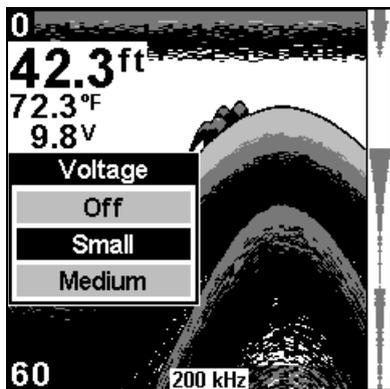
Voltage menu with the voltage display turned off (left) and with voltage set to a small display size (right).
