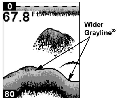
A small amount of Grayline indicates a soft bottom (left), probably sand or mud. More Grayline indicates a harder, rocky bottom (right). Grayline is adjustable. Since Grayline shows the difference between strong and weak signals, adjusting the sensitivity may also require a different Grayline level.
