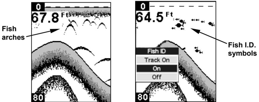
**Underwater scene in normal fish arch mode (left). Fish I.D. menu with the feature turned on (right).**
