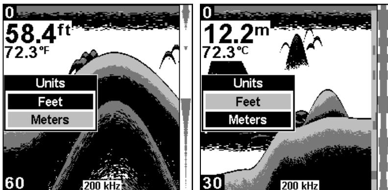
Units set to Feet, which displays temperature in Fahrenheit (left).
