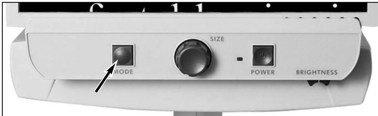
With Merlin LCD Plus turned ON, place a piece of reading material on the X-Y table so that it appears on your monitor at a magnification size that is comfortable for viewing. Follow these steps to program the color select options:
