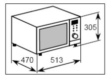
Height: 305 mm Width: 513 mm Depth: 470 mm
