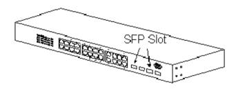
Follow the steps for module adding and removing. [ Add SFP Transceiver ]
