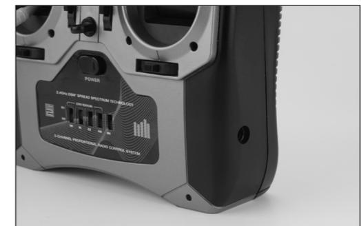
A charging jack is located on the right side of the transmitter. If rechargeable batteries are used they can be conveniently charged without removing them from the transmitter using the charge jack.
