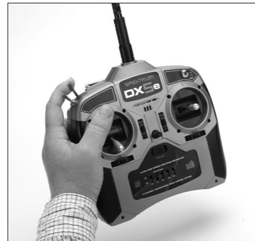
5. Remove the bind plug from the BATT/BIND port on the receiver before you power off the receiver and store it in a convenient place.
