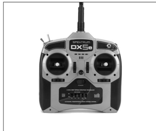
4. Pull and hold the trainer switch on the top of the transmitter while turning on the power switch. Release the trainer switch once the LEDs on the front of the transmitter flash, and a series of tones are heard. Within a few seconds the system should connect. Once connected the LED on the receiver will go solid indicating the system is connected.
